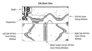
The sonar information from the side-looking beams reveals bottom contour, structure and fish similar to the down-looking beam, but the area covered is to the left and right of the area shown in the down-looking portion, so you actually see more of the bottom. The distance covered by the right and left  $90^{\circ}$  beams is based on the depth setting for the down-looking beam, up to a maximum of 160 feet.
